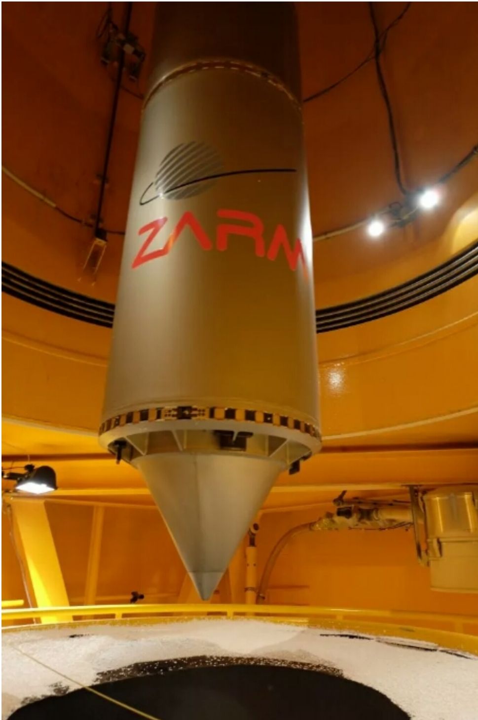
图1：具有实验装置的落塔在自由飞行9.3秒后从减速器中向上提升。图片来源：ZARM Drop Tower Operation and Service Company
