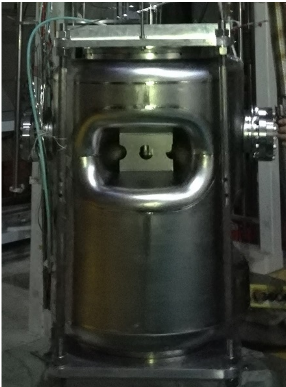
即将进入杜瓦进行垂测的双Spoke腔
